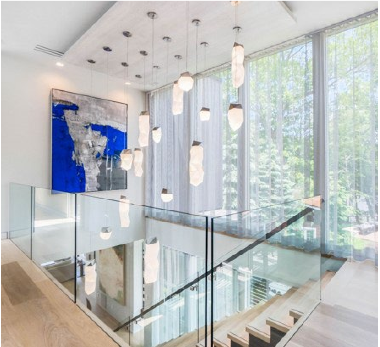
Custom Floor Inset Glass Stair & Guard Rail/Surround: Glass Application: Low Iron; 1/2" Tempered Glass (Required)
